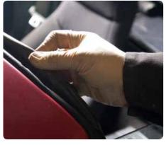
Seal rescue Check all the seals - across the header rail and around the doors, for damage. These need to be sound and clean if they stand an chance of keeping water out and wind noise to a minimum when the hood is up.
