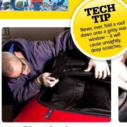
Pivotal point With flexibility restored to the vinyl, gently ease back the roof. Inspect the pivot points of the frame – there are usually plenty of them. Be careful not to catch the hood fabric as you fold the roof back.
