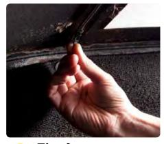
Zip along Next step is to unzip the rear window. Zips can become clogged with dirt, and become very fragile – they're a common cause of hood failure. Don't be tempted to force the zip. Use soapy water to make things easier if required.
