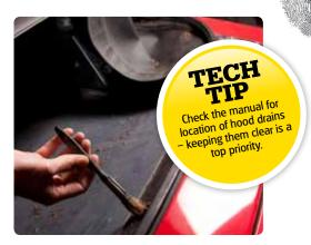
Brush up Work your way around with a soft brush and clean out all the collected debris - it's amazing how much builds up in this area, particularly if the car has been parked up outside for an extended period.
