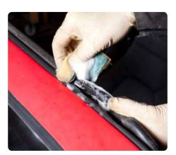
Rubber scrub Clean the seals thoroughly with soapy water, making sure each face of the rubber is clean. Note that the rubbers may involve some kind of rainwater drainage channel, so make sure this is also clear.
