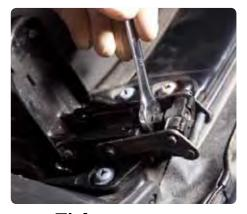
Tighten up It may be necessary to re-tension the hood - but make sure you do this with the hood cool. On the MX-5, it's as simple as tightening the central bolts in the windscreen frame catches.
