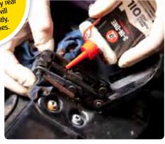
Loosen up Hold a cloth beneath each of the pivot points and add a couple of drops of light oil to each one. Operate the roof through its full arch a couple of times, and makes sure everything is moving freely.
