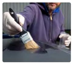
Dry spell When first applied, the proofer appears to 'sit' on the freshly cleaned vinyl. Don't be tempted to rebrush it - as it dries, it sinks in and leaves a pleasing sheen over the fabric of the hood.
