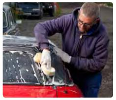
Foam up As per the instructions, we then used a sponge and warm water to work the cleaner into a foam that really lifts the dirt out of the hood. We released the hood clips to work the cleaner right down to the hood base.
