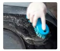
**Brush off** We found that the dirt was so ingrained into our hood that a soft scrubbing brush was needed to work the hood cleaner in, especially along the stitched seams. Don't be too vigorous though.
