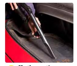
Up the suction Using a vacuum cleaner, work right down into the edges of the hood. Be very careful not to damage the fabric and use the brush for any stubborn debris that will not only hold moisture, but will also push the hood away from the seals.
