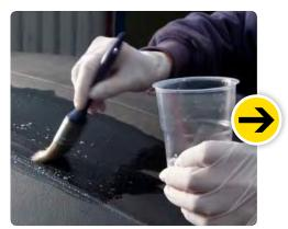
Deep clean The soft top cleaner is brushed on to the vinyl and left for a few minutes to work its magic. Apply an even coat and make sure you get down into those recesses of the hood you've just cleaned out.
