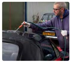
Rinse down Once the whole hood had been worked over, the cleaner was hosed off and it was left to air dry. Again, it's not a bad idea to release the hood to allow the air to circulate right down into the deepest recesses.
