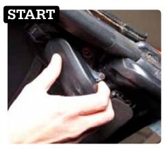
**Under tension** Check your owners manual for the correct way to drop the hood - this usually involves releasing the tension on the roof first. On the Mazda, you release the two clamps on the screen header rail.
