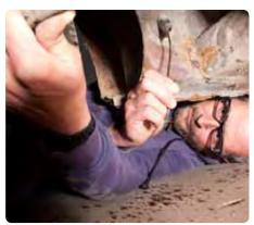
**Drain works** Underneath the car, locate the drain outlets and clean them out - strimmer wire is ideal for this. Blocked hood drains can lead to wet carpets, damaged trim and ultimately, body corrosion.
