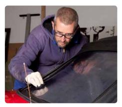
See the light When you feel the cloth starting to drag, it's time to polish up the surface with a clean dry cloth. You'll be amazed at how clear the plastic becomes. A second application may be necessary on long neglected windows.
