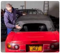
In the fold We're not ready to fold the hood down yet, but gently lift it away from the windscreen header rail to loosen the fabric and allow access to the drainage areas all around the perimeter of the hood.
