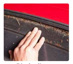
Dig the dirt This is the reason we wanted the window down and out of the way the gutters that run all the way around the base of the hood catch tons of debris. We'll need to remove this before the hood gets wet.
