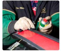
Shiner To protect the rubber and to make it seal more effectively, wipe it over with a silicone spray. Don't forget to treat the door seals, including the joint where the two parts split when the hood folds.
