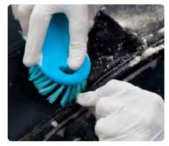
In the gutters The stitched-in gutters above the doors are also mud traps, and if left untreated, the vinyl quickly cracks - we used the scrubbing brush to work along them and clean them out.
