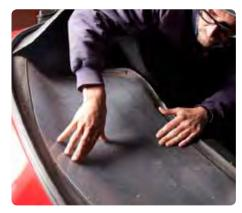
Plastic weakness Lay the window flat. Plastic rear windows are another weak point and are easily scratched or cracked, especially when they're dirty or untreated.
